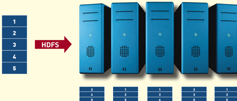
HDFS breaks incoming files into blocks and stores them redundantly across the cluster.
