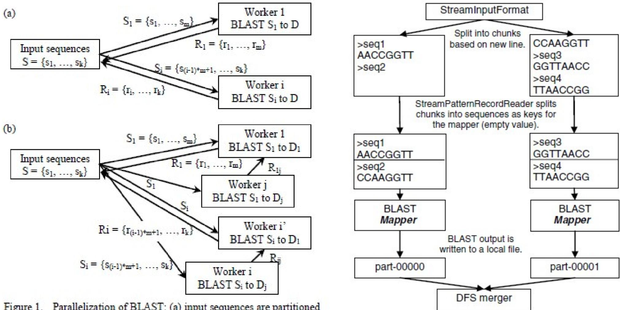
Figure 1. Parallelization of BLAST: (a) input sequences are partitioned
